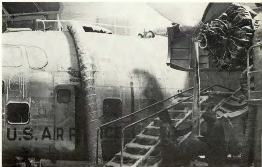
B-r-r-r-r, it's cold! F-100 and C-123 undergo cold weather testing in Air Force's climatic hangar at Eglin AFB. Temperature in hangar may range from 165°F. down to -65°F.
