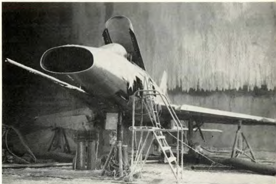
B-r-r-r-r, it's cold! F-100 and C-123 undergo cold weather testing in Air Force's climatic hangar at Eglin AFB. Temperature in hangar may range from 165°F. down to -65°F.
